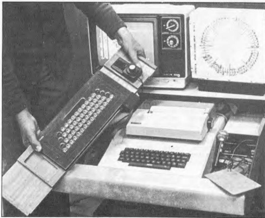
The TASA (Touch Activated Switch Array) touch keyboard with transparent perspex overlay to guide unsteady hands or head-mounted probes through gaps to the keys.
